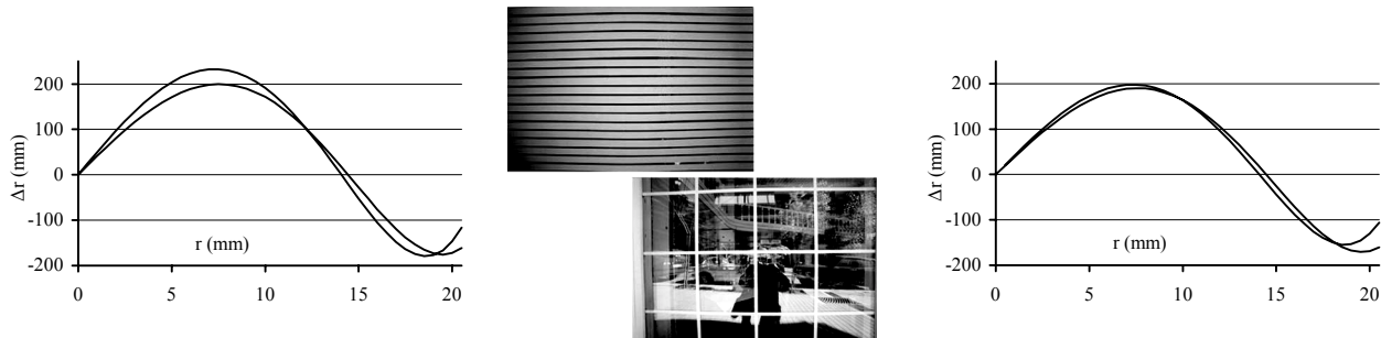
Figure 10: Distortion curves for two images of the same lens from line-fitting and from fitting to partial rectification residuals
