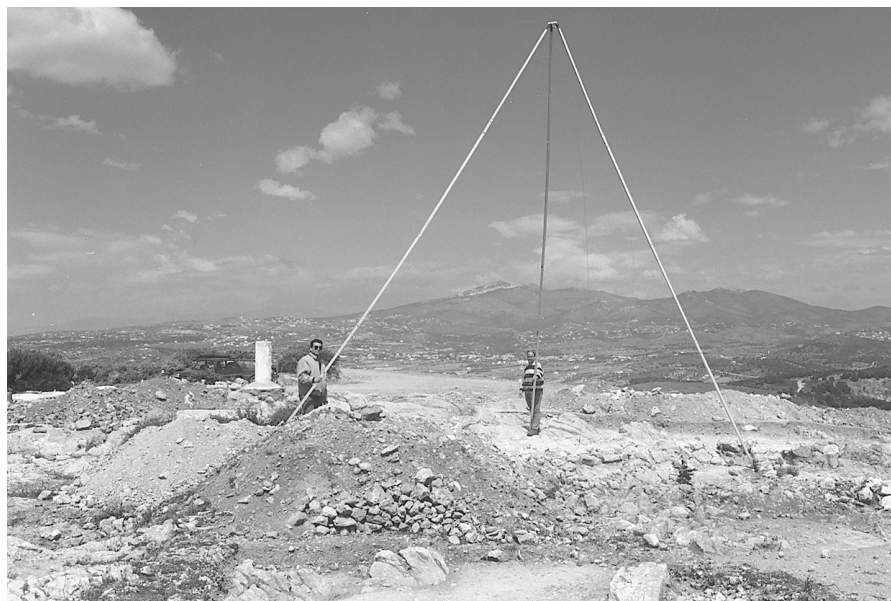
FIG. 5. The special tripod for low altitude photography.
