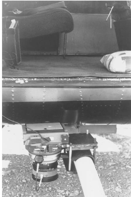
FIG. 2. The Wild P31 camera mount on the helicopter skid.
